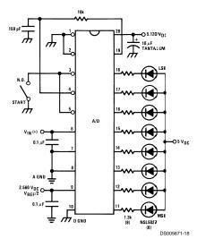
FIGURE 9. Basic A/D Tester
