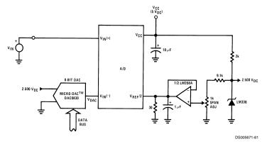
$$\begin{split} &V_{REF}/2\text{=}128 \text{ mV}\\ &1 \text{ LSB=1 mV}\\ &V_{DAC}\text{\le}V_{IN}\text{\le}(V_{DAC}\text{+}256 \text{ mV})\\ &0\text{ \le}V_{DAC}\text{ < }2.5\text{V} \end{split}$$
