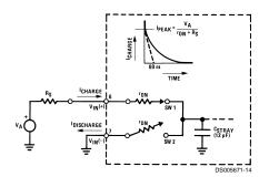
$r_{ON}$  of SW 1 and SW 2  $\cong$  5  $k\Omega$   $r=r_{ON}$   $C_{STRAY}$   $\cong$  5  $k\Omega$  x 12 pF = 60 ns
