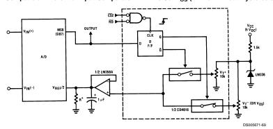
\*See Figure 5 to select R value DB7="1" for  $V_{IN}(+)>V_{IN}(-)+(V_{REF}/2)$  Omit circuitry within the dotted area if hysteresis is not needed
