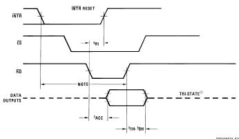
Note: Read strobe must occur 8 clock periods (8/f<sub>CLK</sub>) after assertion of interrupt to guarantee reset of  $\overline{\text{INTR}}$  .
