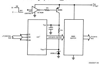
\*Use ADC0801, 02, 03 or 05 for lowest power consumption. Note: Logic inputs can be driven to  $V_{CC}$  with A/D supply at zero volts. Buffer prevents data bus from overdriving output of A/D when in shutdown mode.
