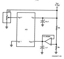
$\mu P$  Compatible Differential-Input Comparator with Pre-Set  $V_{OS}$  (with or without Hysteresis)
