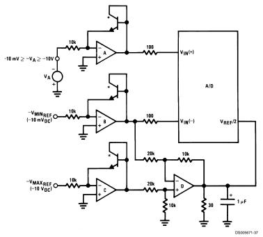
\*LM389 transistors A, B, C, D = LM324A quad op amp
