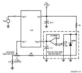
Span Adjust: 0V  $\leq$   $V_{IN} \leq$  3V
