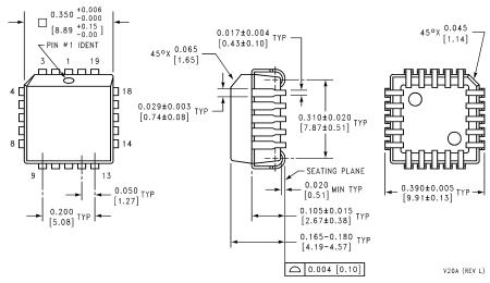
Molded Chip Carrier Package (V)
