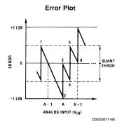
FIGURE 3. Clarifying the Error Specs of an A/D Converter Accuracy=±½ LSB
