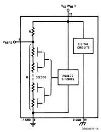
FIGURE 6. The  $\mathbf{V}_{\text{REFERENCE}}$  Design on the IC
