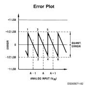
FIGURE 1. Clarifying the Error Specs of an A/D Converter Accuracy=±0 LSB: A Perfect A/D
