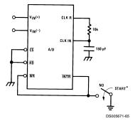
\*After power-up, a momentary grounding of the  $\overline{\mbox{WR}}$  input is needed to guarantee operation.
