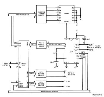
FIGURE 19. Microprocessor Interface Circuitry for Differential Preamp
