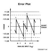
FIGURE 2. Clarifying the Error Specs of an A/D Converter  $Accuracy=\pm \frac{1}{4}$  LSB
