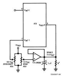
\*Add if  $V_{REF}/2 \le 1 \ V_{DC}$  with LM358 to draw 3 mA to ground.
